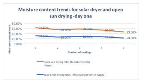
Figure 3 moisture content rate trends for solar dryer and open sun drying for day one
