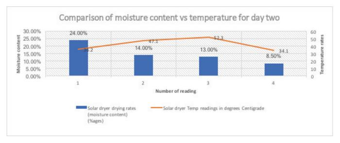
.Figure 9 comparison of moisture content and temperature rates of day two readings
