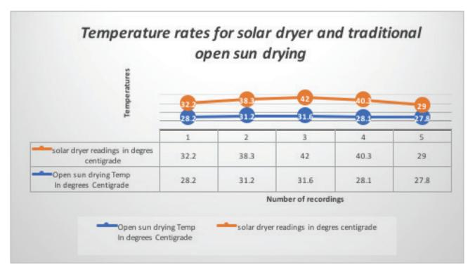
Figure 2 Temperature rates for solar dryer and traditional open sun drying day one
