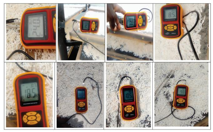
Figure 4 of the sample recording show the performance of cassava chips in the solar dryer which on the second day started reading at 10:00am with moisture content of 24.0% to 8.5 % for samples in the solar dryer.
