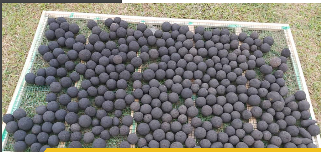
Display of the final product of fuel briquettes which are left to dry in an open ground, this is to make the briquettes more solid.
