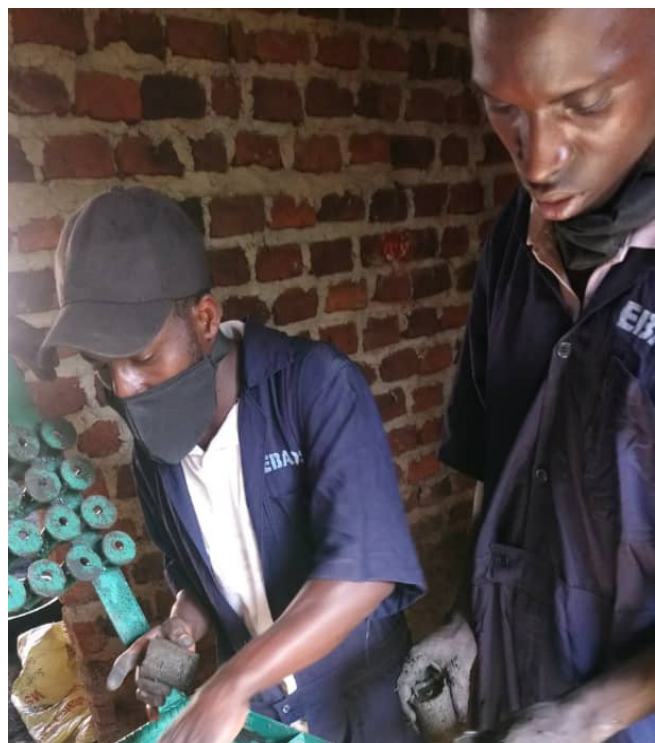
Youth using briquettes making machine to cut them into shape so that they are easy to transport and carry. The machine does all the work of shaping the briquettes into more manageable form.
