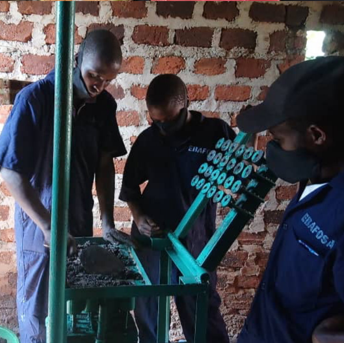
A demonstration of the youth making briquettes from cassava wastes during one of the trainings undertaken by EBAFOSA Uganda to showcase the adoption of alternate source of energy that conforms to clean energy standards.
