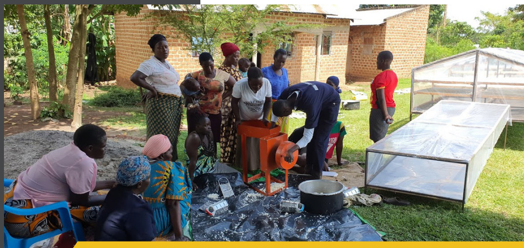
An innovative volunteerism actor demonstrates how to chip cassava using a chipper for drying the cassava using solar dryers showcasing no pollution from the process
